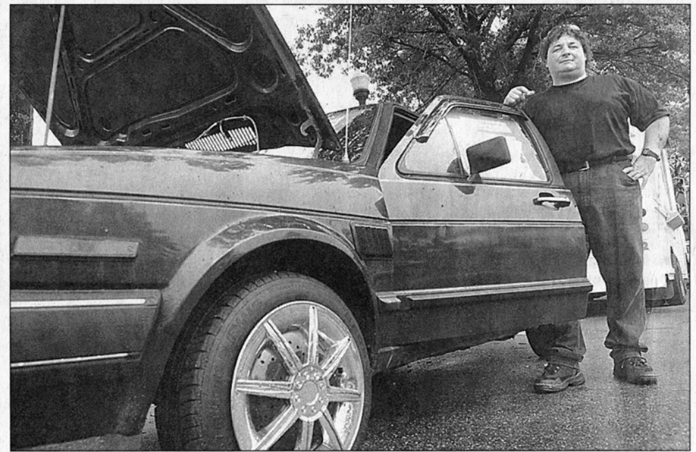
BURNS OIL, AND THAT'S JUST FINE: Virgínio Mendonça with his 1986 Volkswagen Jetta, a diesel model that he modified to run on used vegetable oil. The car gets 44 miles per gallon and has been running for six months with no problems.
